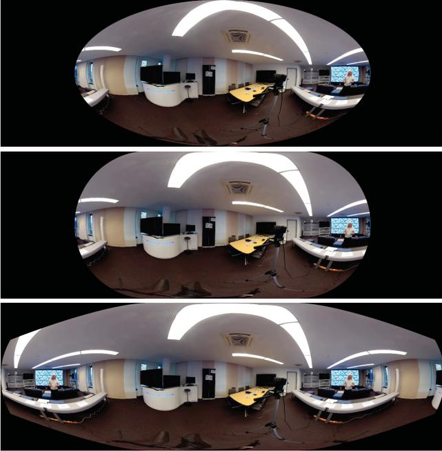
Fig. 1. Example of Mollweide projection (top), hybrid Mollweide projection ( $\alpha = 0.5$ , middle) and hybrid Mollweide projection with border ( $\alpha = 0.5$ , border=0.125, bottom).
