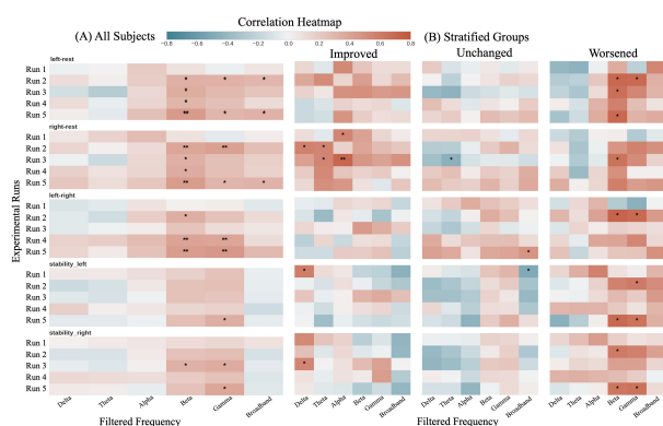
Figure 3: Spearman correlation heatmaps between expected MI-BCI performance and neural metric values across frequency bands for a) all subjects and b) behavioral groups. Positive correlations indicate association with higher expected MI-BCI performance. Color intensity indicates correlation strength (Red = Positive, Blue = Negative). Asterisks denote significance (* p < 0.05 , ** p < 0.01 ).
