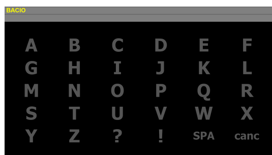
Figure 1: P300-speller 5x6 matrix used for the stimulation protocol. A row or column intensifies for 120 ms every 120 ms. The word at the top of the window is the text to be spelled.
