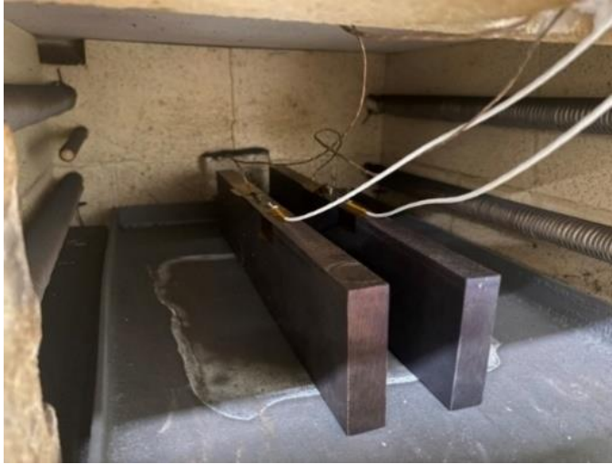
Fig. 4 Substrates with installed strain gauges in chamber furnace
