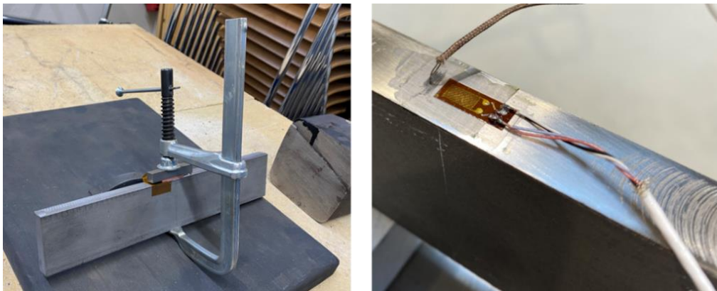
Fig. 3 Mechanical clamping for curing under pressure (left), installed gauge and thermocouple (right)
