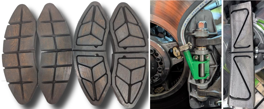
Figure 2: From Left to right, original DBU pad, modified DBU pad, modified DBU pad holder, modified TBU sole.
