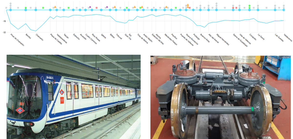
Figure 4: Track profile (upper); 2000-series operated on L1(left); bogie configuration (right).
