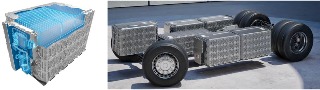
Figure 4: left – Battery pack layout, right- arrangement of battery packs on a MAN truck [5]
