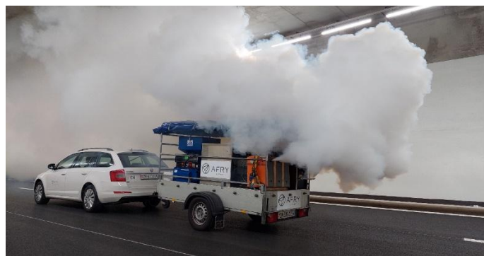
Figure 1: Experimental setup with smoke generators on trailer
