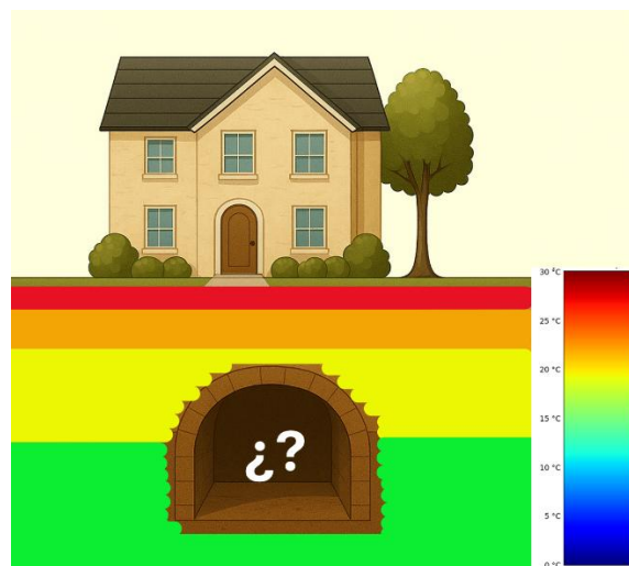
Figure 2: Thermal equilibrium will depend on the external, geothermal and ventilation conditions of the tunnel.
