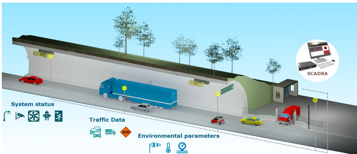
Figure 1: Smart Tunnel with SCADRA
