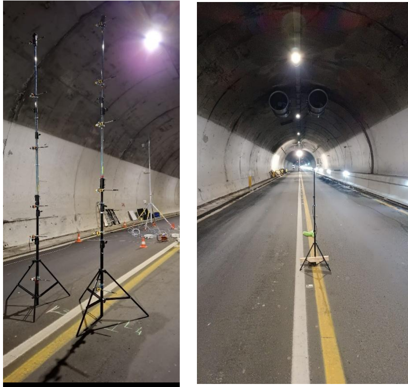
Figure 5: Tripod set-ups for velocity measurements (left) and pressure measurements (right)
