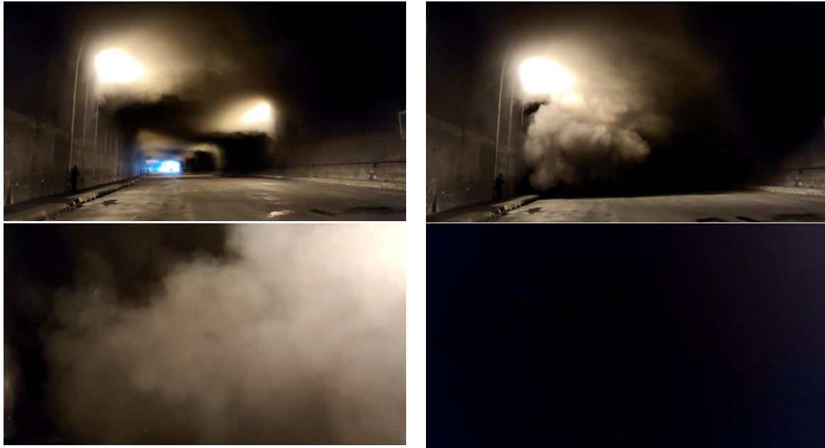
Figure 1: Smoke layer on a real test at TST. From left to right and up to down: an instant before the ventilation activation; 5 seconds after; 10 seconds after; 15 seconds after
