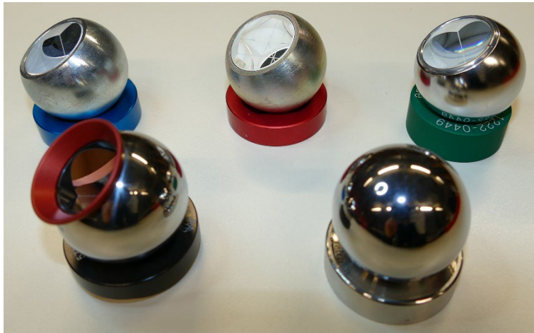
Fig. 1: Spherical glass-body reflectors of the investigated lots and higher-order references. Back: An uncertified 1445 reflector is mounted on a blue drift-nest, a certified 1445.SN reflector on a red drift-nest, and an uncertified 1448 reflector on a green drift-nest. Front: The glassless reference SMR is a red-ring reflector and mounted on a black drift-nest, while the reference steel ball is mounted on a silver drift-nest.
