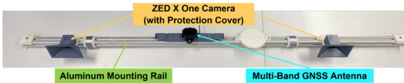
Fig. 2: System integration on the aluminum mounting rail.
