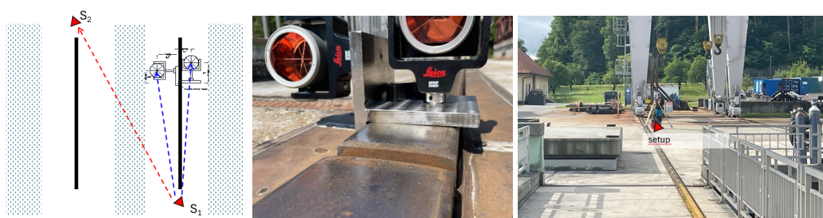
Fig. 1: The principle of measuring crane rail tracks
