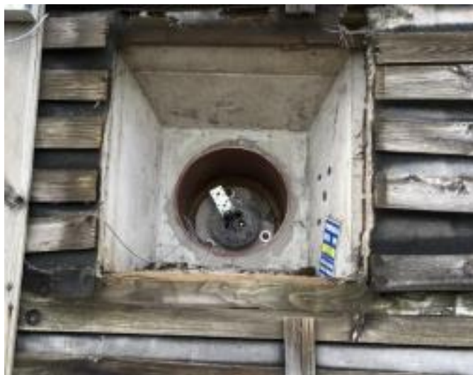
Figure 5: Upgrade of existing extensometer for 24/7 and online measurement.
