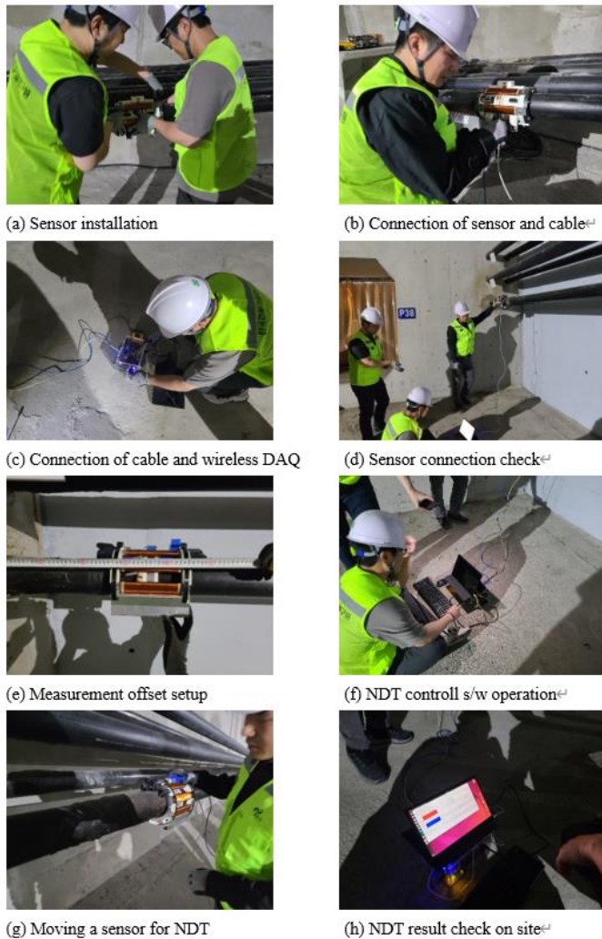
Figure 7. NDT process of TFC-based EM sensor
