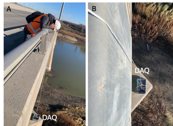
Figure 2. A) The data acquisition device on a bridge pier cap. B) View from the bridge deck of the DAQ system sitting on the pier cap.
