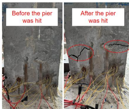
Figure 5. Comparative analysis of damage at the base of bridge piers
