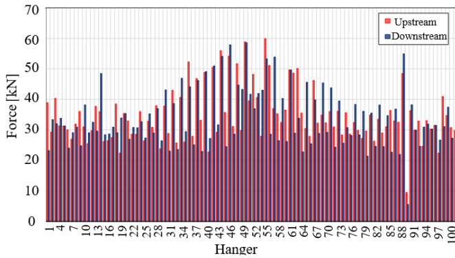
Figure 5. Calculated force values in the hangers on the upstream and downstream side of the bridge
