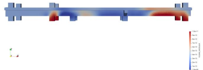
Figure 19. Overfitted material parameters. Young's modulus of concrete reaches upper and lower bounds.
