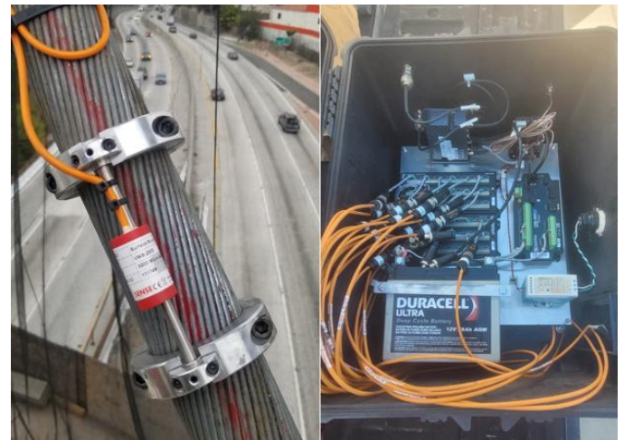
Figure 4. Strain Gauge assembly and logger setup.
