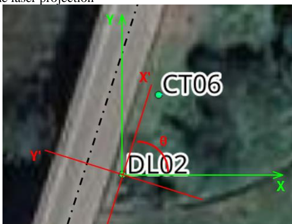
Figure 12. Axis diagram for the sensor DL02
