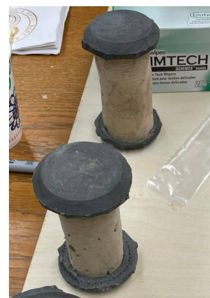
Figure 8. Adobe specimens with sulfur caps
