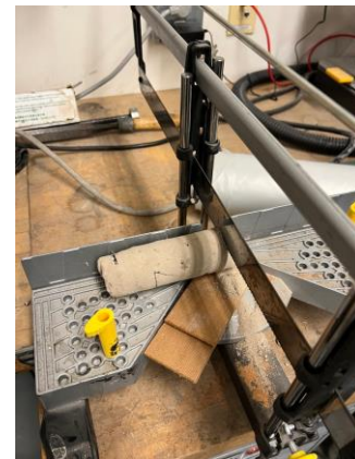
Figure 7. Adobe specimen in a cutting device
