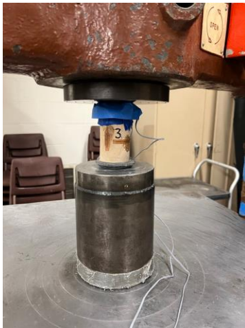
Figure 10. Adobe specimen in the compression test machine.
