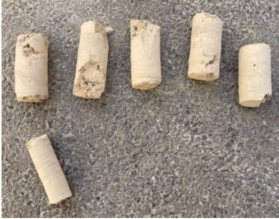
Figure 5. Collected specimens before cutting them to the same length and selecting the best ones
