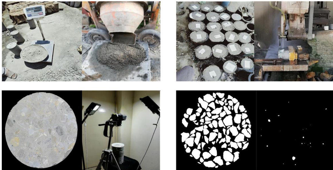
Figure 1. Preparation of Concrete Mixtures (Top Left), Casting and Cutting of Samples (Top Right), Image Acquisition (Bottom Left), Image Labeling (Bottom Right).
