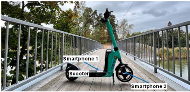
Figure 1. Scooter with two smartphones.
