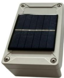
Figure 6. Solar-powered gateway (Copyright: Christian Steffes, Infrasolute).
