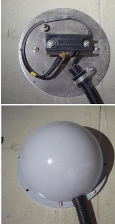
Figure 4: First approach for a sensor mounting device including protection cover [5]
