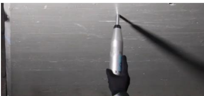
Figure 2: HSU-Nielsen source (0.5mm) to verify the sensor mounting quality (top).
