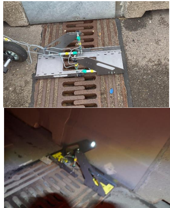
Figure 6. Midspan joint custom displacement sensor
