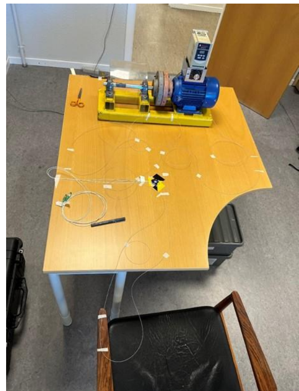
Figure 6. The vibrating test rig during a bench test, with a FBG chain and FGB rosette located on the table.
