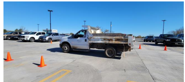
Figure 2. The truck on the slab in a static load test.
