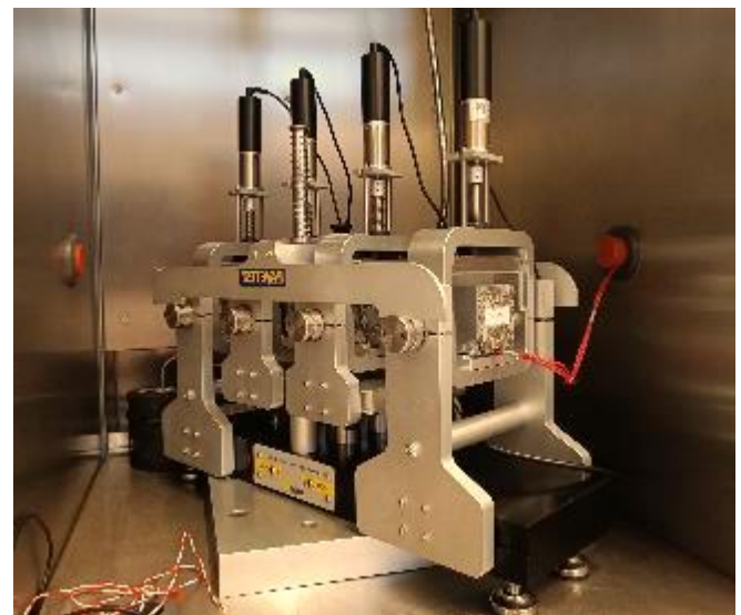
Figure 2. Four-point bending setup for fatigue test.
