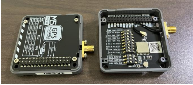
Figure 3. M5Stack GPS V2 module: (left) Top View, and (right) Bottom View
