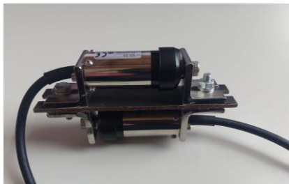
Figure 5. Crack displacement transducers on a steel plate.
