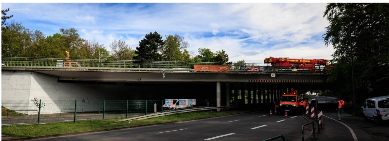
Figure 10: Bridge during load test with 48t mobile crane
