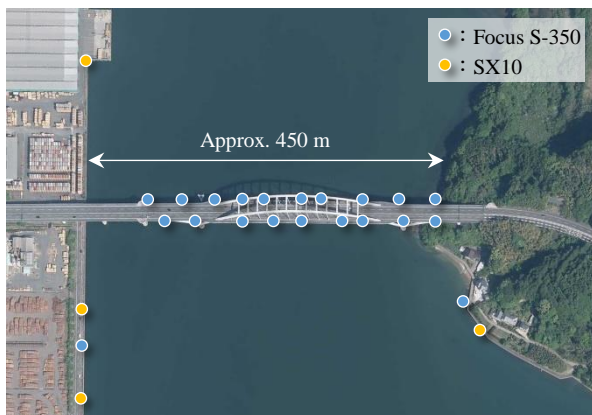
Figure 13. Positions of measurements by TLS (Created using aerial photographs (by the Geospatial Information Authority of Japan))
