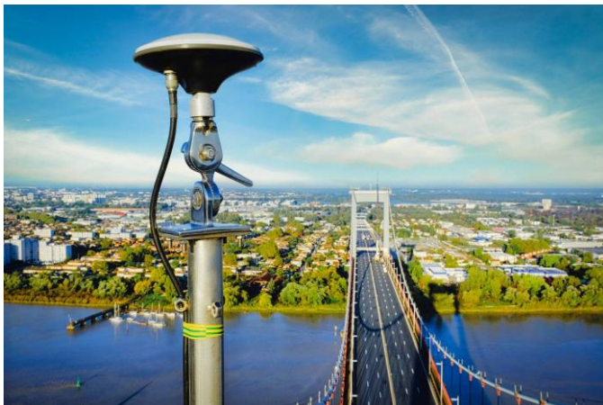
Figure 5. GNSS antenna installation on the 90-meter-high pylon of the Aquitaine Bridge in Bordeaux, France.
