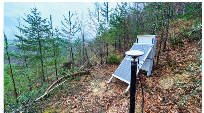
Figure 11. GNSS antenna connected to an autonomous TEXTant ® station powered by a solar energy system.
