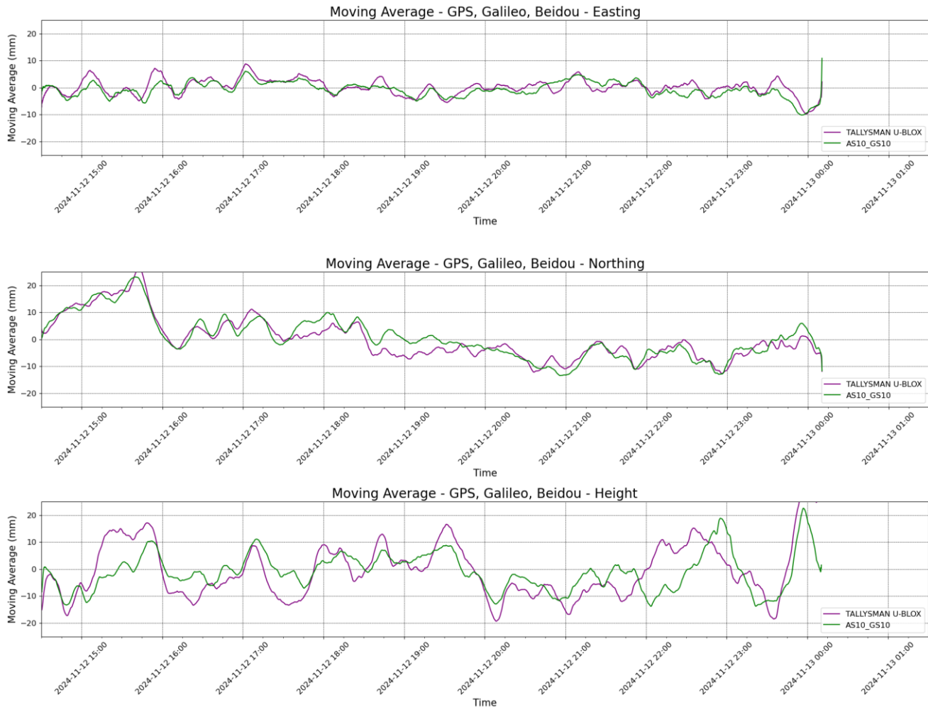
Figure 11: Moving average variation of the low-cost system and fully geodetic system.
