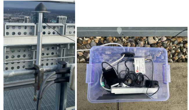
Figure 9: Tallysman TWI antenna connected to the handrail of the building rooftop. Right- U-blox F9P receiver connected to the antenna and Raspberry Pi device to log the data.
