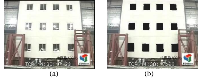
Figure 3. An Example for structural RoUs identification based on TL (a) original frame (b) processed frame
