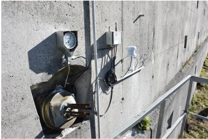
Figure 8. Digitization of an already installed anchor load plate.
