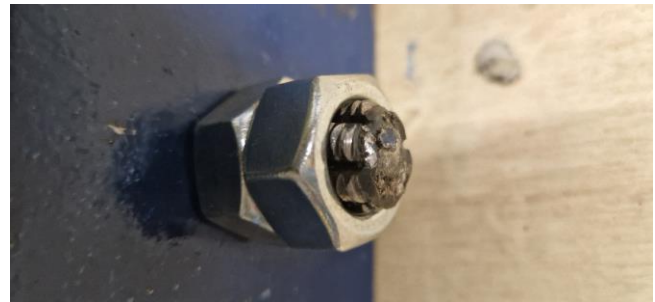
Figure 13. External thread used for the application of a threaded nut on an anchor strand.
