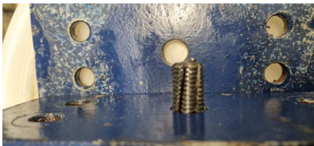
Figure 12. External thread retrofitting to a pre-stressed anchor strand.
