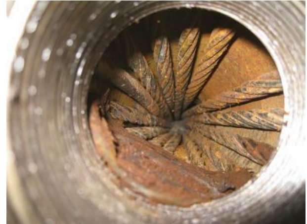
Figure 5. Corroded strands within the anchor head area.
