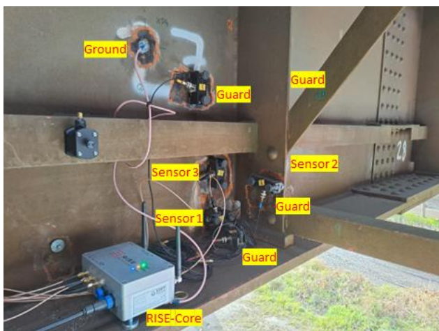
Figure 5 AE sensor arrangement at the monitored position with suspected crack. Sensor 2, not in the picture, is positioned behind the connection detail in the distance of 12 cm from the suspected crack.
