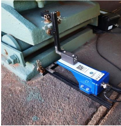
Figure 6. A 6D sensor installed on a roller bearing of a railroad bridge
