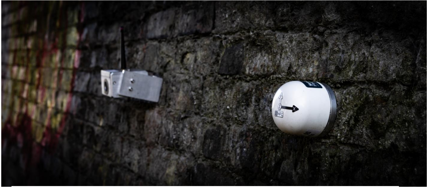
Figure 2: Wireless Sensor Nodes: 3-Axes-Tilt-Sensor (Triaxial Tilt Sensor) (Foreground) and Laser Distance Sensor (Background)
