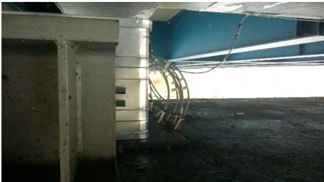
Figure 7. Measuring system on the bearing shelf/seat of the abutment.
