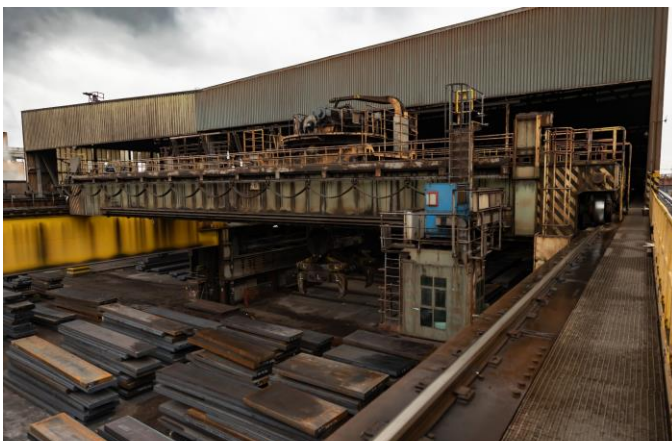
Figure 8: Mobile crane bridge with centrally positioned gateway
