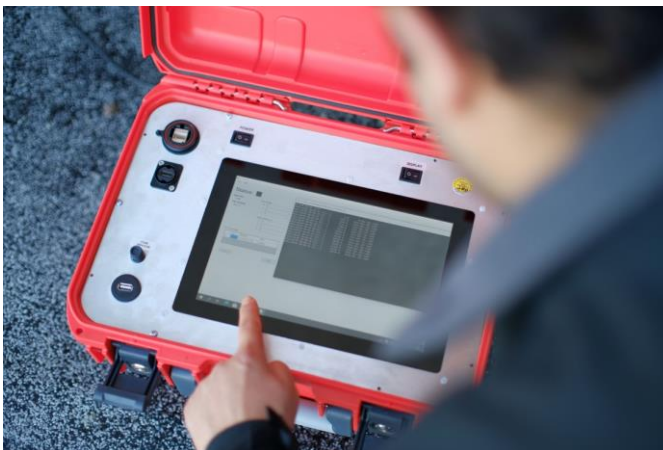
Figure 2. TEXtant ® GNSS station initiating autonomous operation and data processing upon activation.
