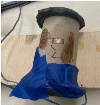
Figure 9. Adobe specimen with bi-axial strain gage.
