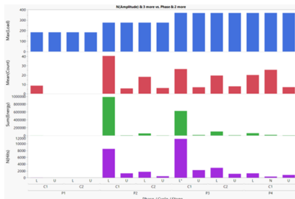
Figure 10: Maximum loads (Max - blue), and number of hits (N - purple), total energy (Sum - red) and mean count (Mean - green) of the hits for individual phases (P1, P2, P3), cycles (C1, C2) and stages (loading L and unloading U).
