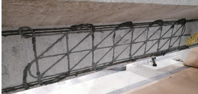
Figure 1. 2D sensor arrangement for shear monitoring
