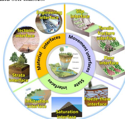
Figure 1 Schematic diagram of rock and soil disasters and the three types of interfaces.
