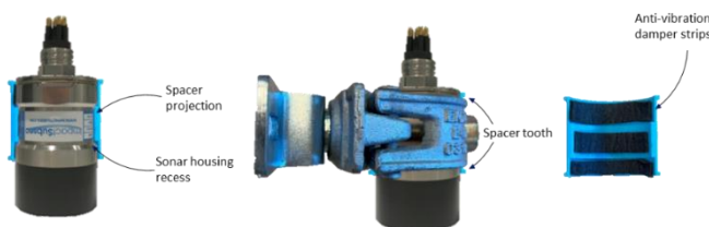
Figure 7. Detailed parts of the spacer
