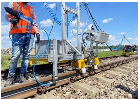
Figure 8. Semi-automatic rail cart used for sensors' effective installation along the rail.
