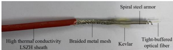
Figure 3. Structure of the DTS temperature-sensing cable: (a) Schematic diagram; (b) Physical photograph.
