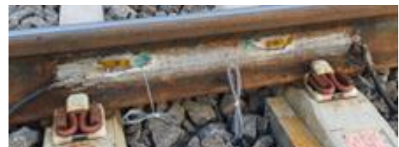
Figure 6. Full Wheatstone bridge mounted on the neutral axis of the rail web
