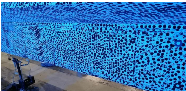
Figure 5. DFOS grid covered with DIC speckle pattern
