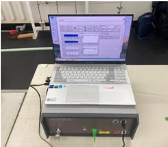
Figure 2. PNC-OFDR based distributed strain analyzer and a laptop PC for data processing.
