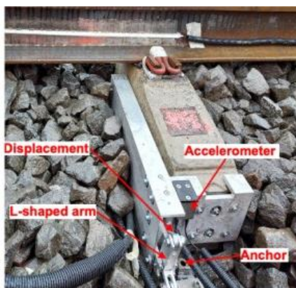
Figure 9. Detail of an instrumented sleeper equipped with a vertical base plate, an L-shaped mechanism, one accelerometer and one displacement transducer.
