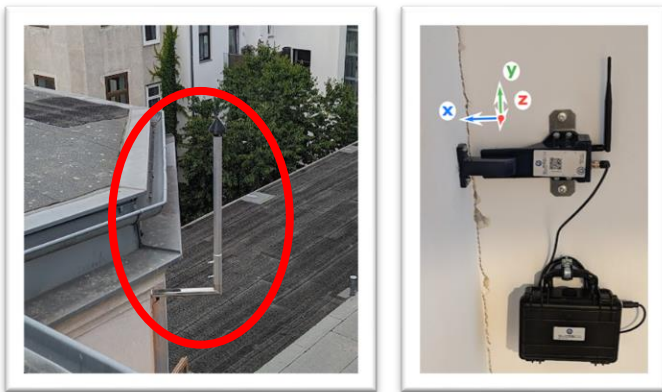
Figure 10. Left: Mounted GNSS antenna on the exterior wall of the residential building. Right: 6D sensor mounted in a building corner near the GNSS antenna.
