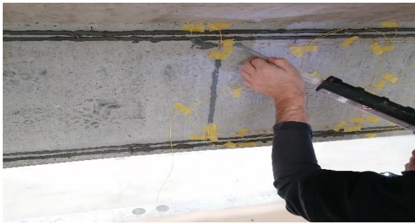
Figure 4. Sensor bonding procedure on concrete
