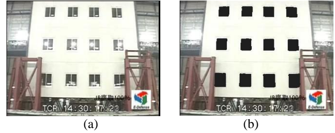
Figure 3. An Example for structural RoUs identification based on TL (a) original frame (b) processed frame
