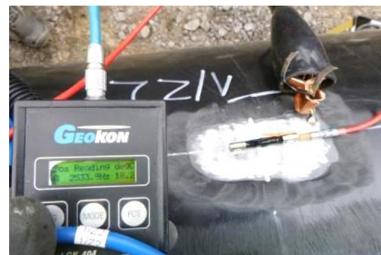
Figure 15. Vibrating wire gauges and their initial check during installation on the pipeline section.
