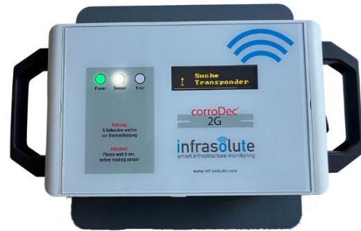
Figure 7. IoT handheld reader for manual sensor data acquisition (Copyright: Christian Steffes, Infrasolute).
