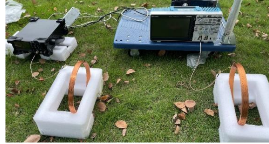
Figure 3 Outdoor Transmission Experiment Platform for Magnetic Induction Signal Using Mutual Inductance Coils
