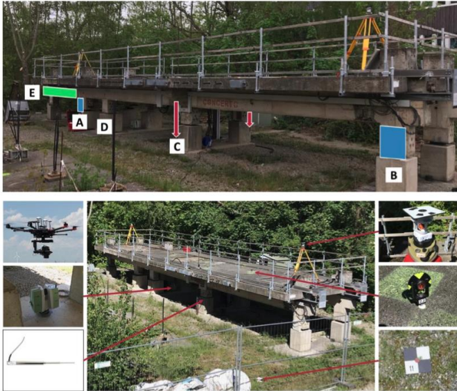
Figure 11. Experimental Bridge "Concerto". Upper part: indication of support (A, B), ground anchor (C), Deformation transducer positions (C and D), and cantilever arm (E). Lower part: instruments (UAV, laser scanner, and transducer) and signalization of reference points [5].
