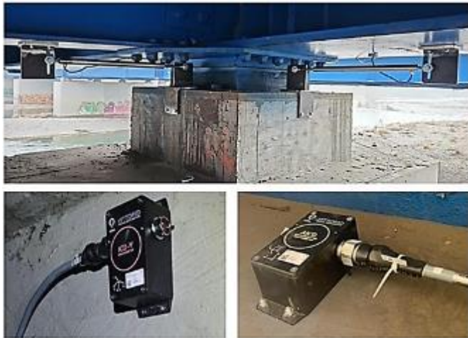
Figure 3. Discrete sensors used: displacement transducers (top), biaxial inclinometer (bottom left), triaxial accelerometer and biaxial inclinometer (bottom right).
