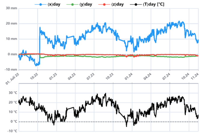
Figure 2. Measurement data for monitoring a roller bearing: effects of unintended displacements during maintenance work and wildlife damage
