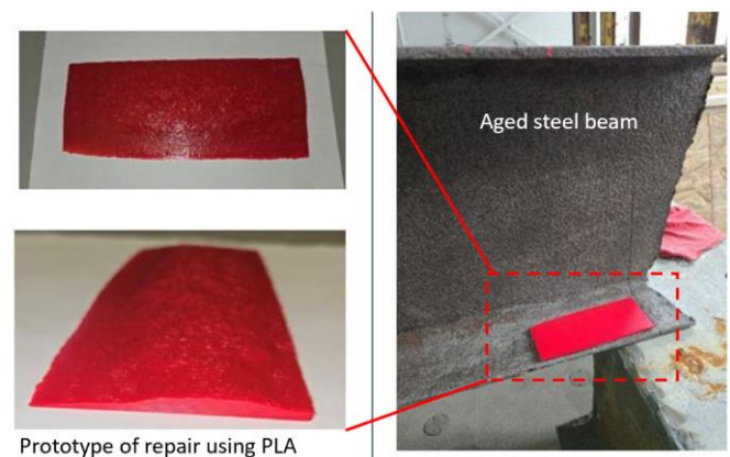
Figure 4. Reconstruction of bottom flange of aged steel beam using different number of images.
