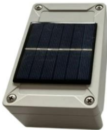
Figure 6. Solar-powered gateway (Copyright: Christian Steffes, Infrasolute).
