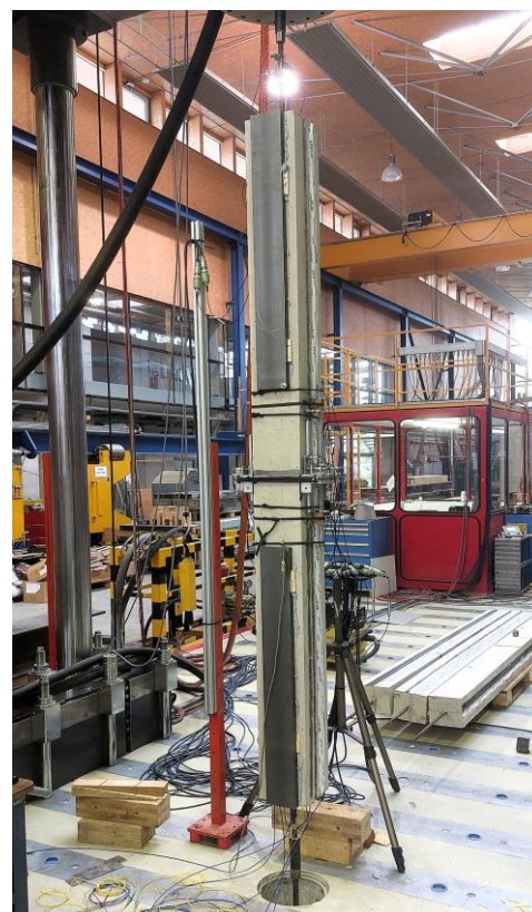
Figure 1. Practical realization of laboratory test setup with one defined crack location.
