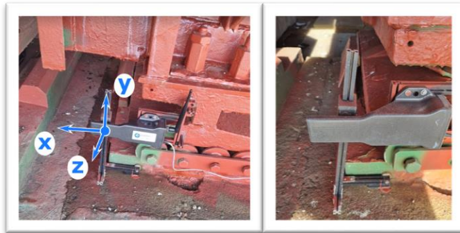
Figure 1. Images of the Monitored Roller Bearing: Left: Condition at installation with corresponding axes; Right: Sensor after maintenance work, displaced and sandblasted
