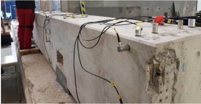
Figure 1: Evaluation of several AE sensors on a concrete beam to investigate the capability to detect wire breaks
