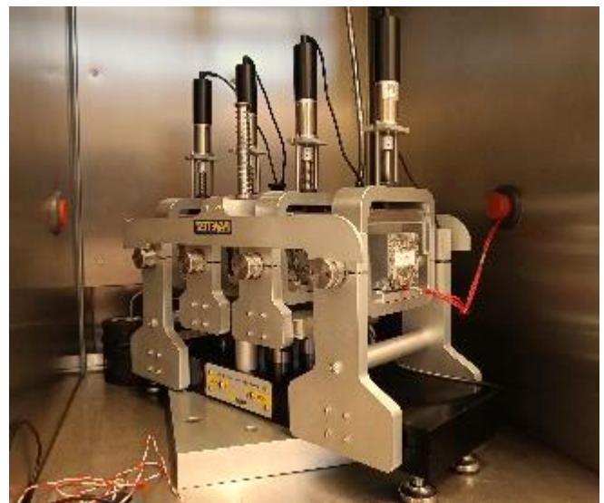
Figure 2. Four-point bending setup for fatigue test.
