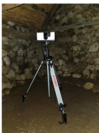
Figure 9: Artec Ray scanner in operation in the kitchen of Keldur.
