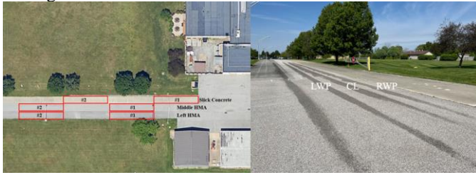
Figure 16. The test fields: three track roads in INDOT. Each road includes two longitudinal sections (left) and three transversal locations (right).
