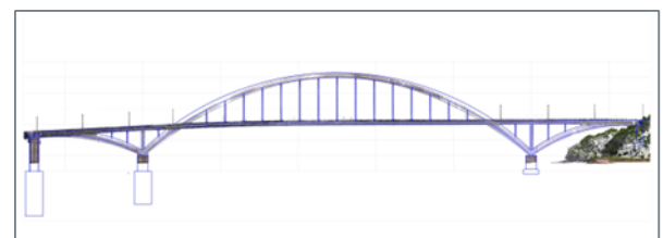
Figure 15. Overlay of measured cloud point data and drawing data
