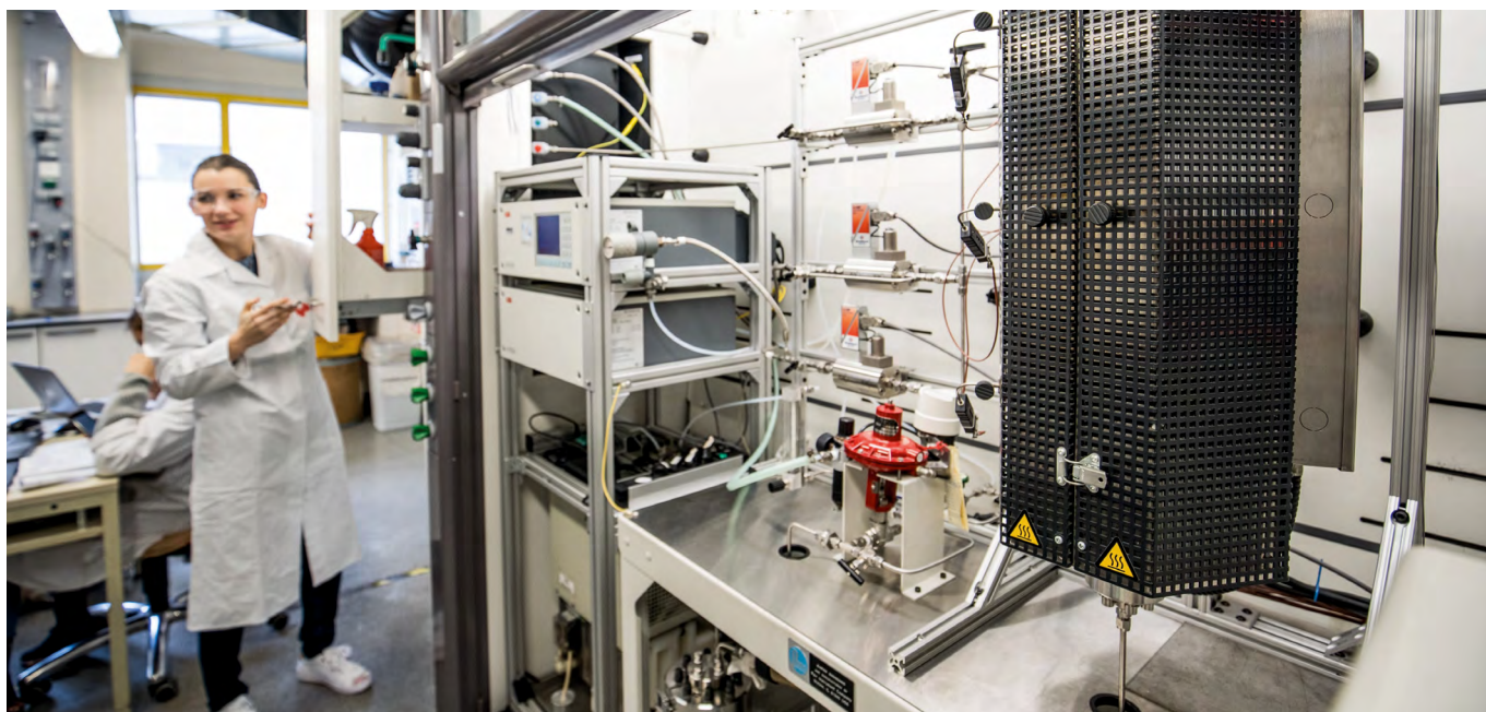
↓ Figure 3: Test stand for heterogeneous gas-phase reactions at the Institute of Chemical Engineering and Environmental Technology.
