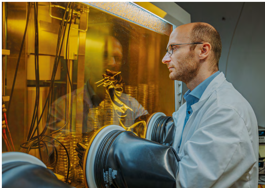
↑ Figure 1: Thomas Rath at the Institute for Chemistry and Technology of Materials working in a glovebox, where perovskite solar cells are fabricated and characterized.
