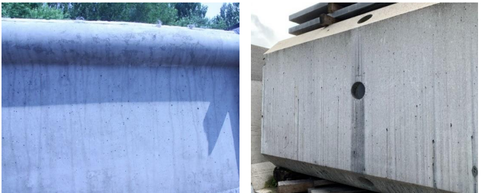
Figure 4.1 UHPC surface with air pores
