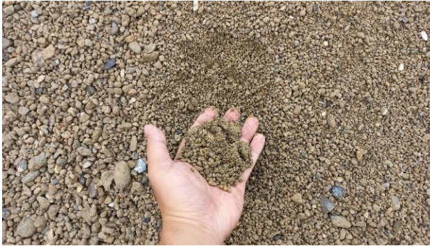
Figure 5.7 Photo of the used RCA
