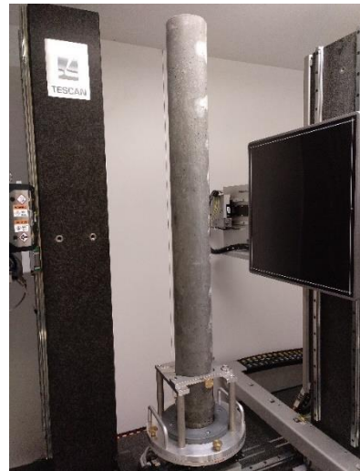
(b) \Phi 100 \times H 1000 \text{mm}^3 column
