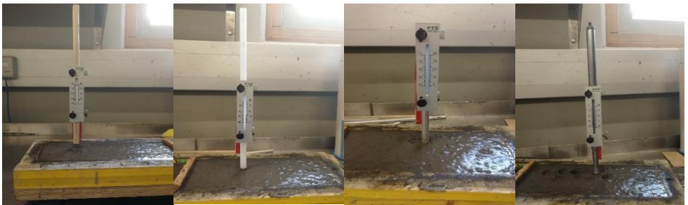
Figure 3.7 Test photos of the surface resistance of the “elephant skin” using the Vicat apparatus
