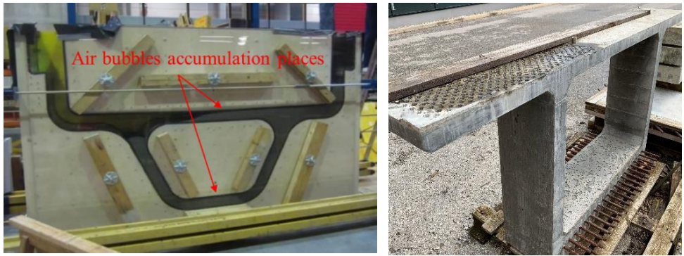
Figure 4.2 Air bubbles accumulate in a specific position in an enclosed formwork
