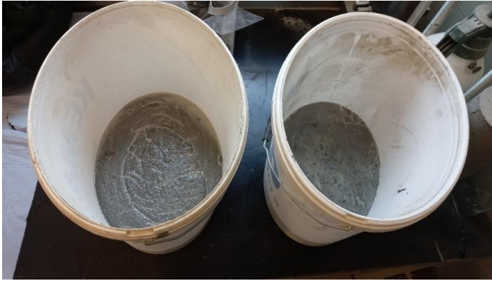
Figure 4.50 UHPC mixtures stored in the open buckets for 90min of the de-airing process
