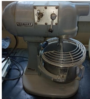
Figure 2.4 Small Hobart mixer (5L)
