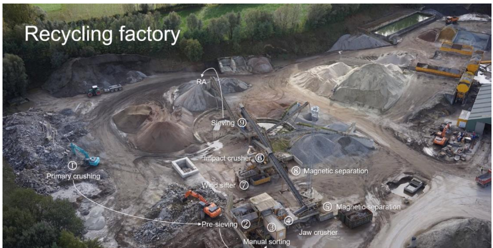
Figure 5.1 Production of RCAs in a recycling factory ( http://www.obbc.be/nl/installaties )
