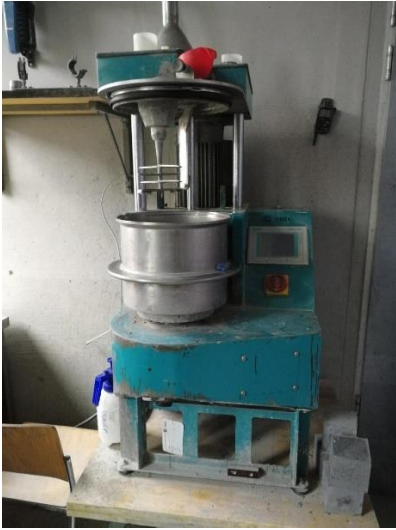
Figure 2.2 Eirich R01 mixer (10L)
