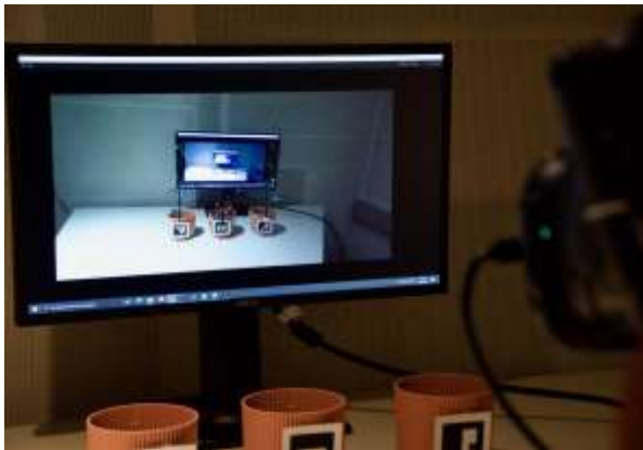
Figure 1: The used AR-Set-up with the HTC Vive Pro and attached ZEDmini stereoscopic camera. On the table one can see the plant pots and the screen shows the virtual plants that the participant is seeing via the VR-goggles.
