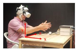
Figure 2: The experimental setup with Meta Quest 2 placed over the EEG cap. The axes represent the coordinate frame of recorded movement trajectories.
