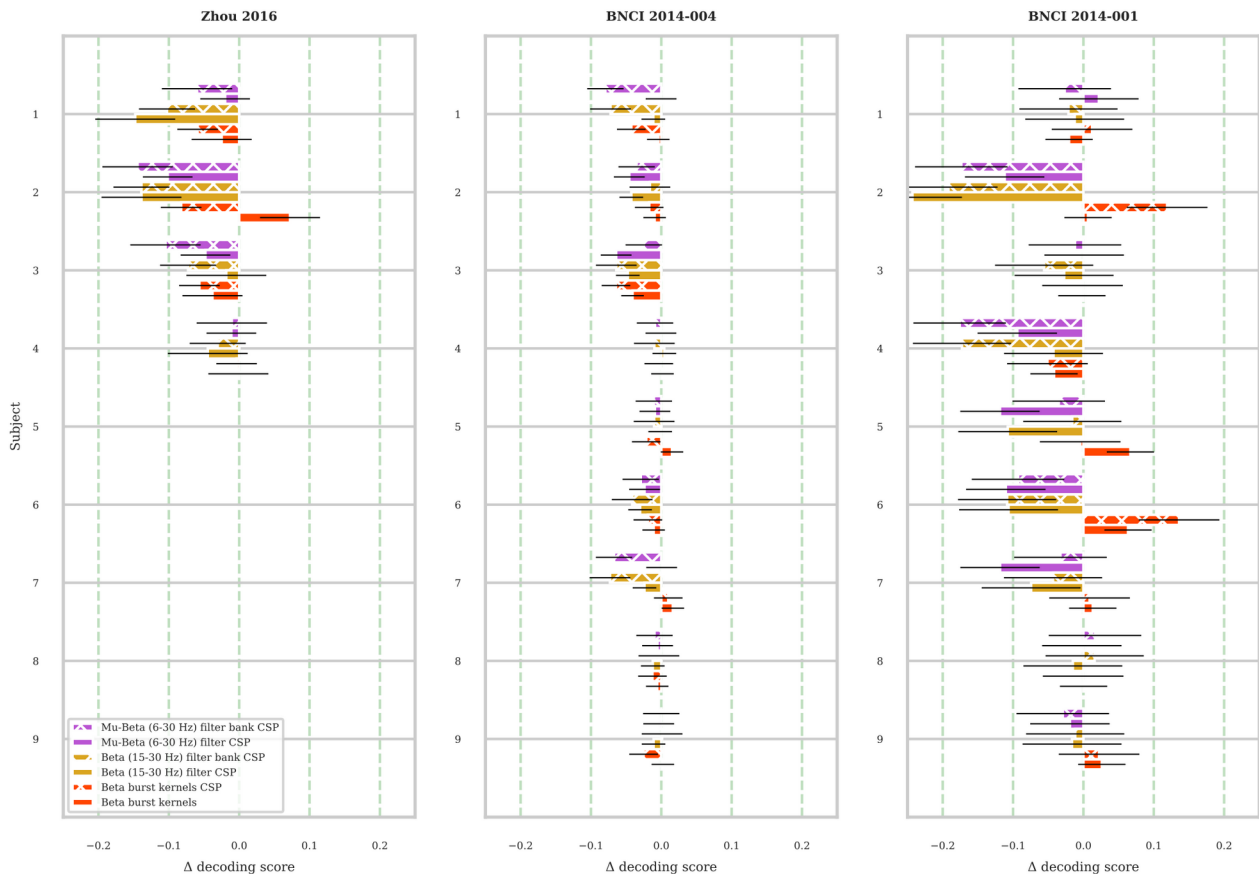
Figure 2: Average difference in decoding score (area under the curve of the receiver operator characteristic) between classification score of a transfer learning session and classification score obtained using all available trials per subject. A value of 0 indicates no difference in decoding between the two approaches. Positive values or negative values indicate a performance gain or loss respectively when adopting a transfer learning approach.
