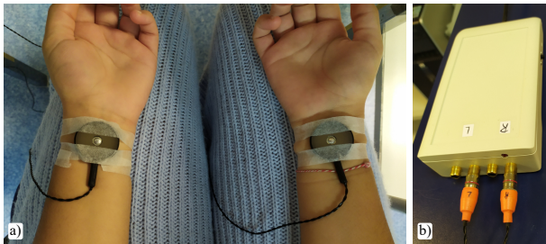
Figure 2: (a) C-2 factors were taped on the left and right wrists. (b) Stimulation box: a micro-controller establishes the connection to the computer and powers the factors.
