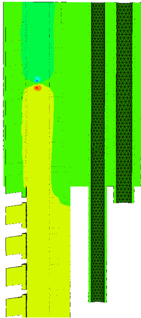
Figure 4: Visualization of the potential field distribution inside the model for an axially oriented electric dipole located in the spinal cord.
