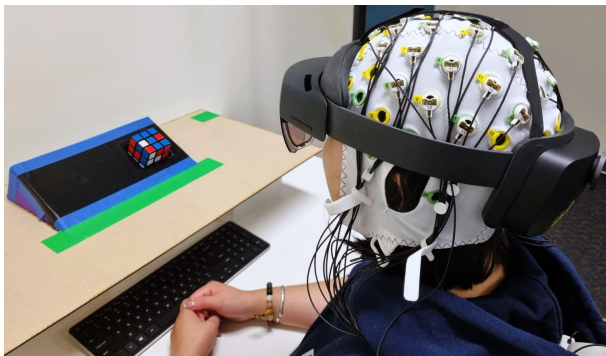
Figure 1: Experimental setup. A participant wearing an EEG cap and an HMD. The tricolor Rubik's cube is in its starting position.
