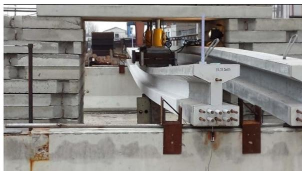
Figure 3 Deflection of the pretensioned UHPC beam under testing load
