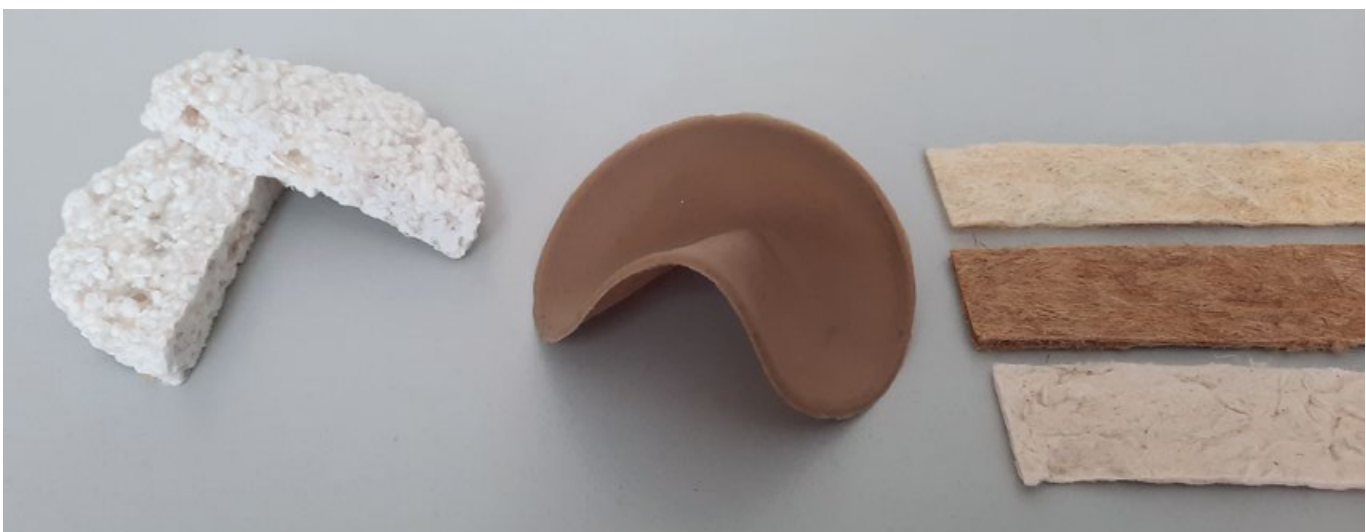
Figure 3: Alginate composite with a porous structure offers an alternative to the standard thermal insulation structure (left), the elastic alginate-clay material (center) and alginate-fiber composite (right)
