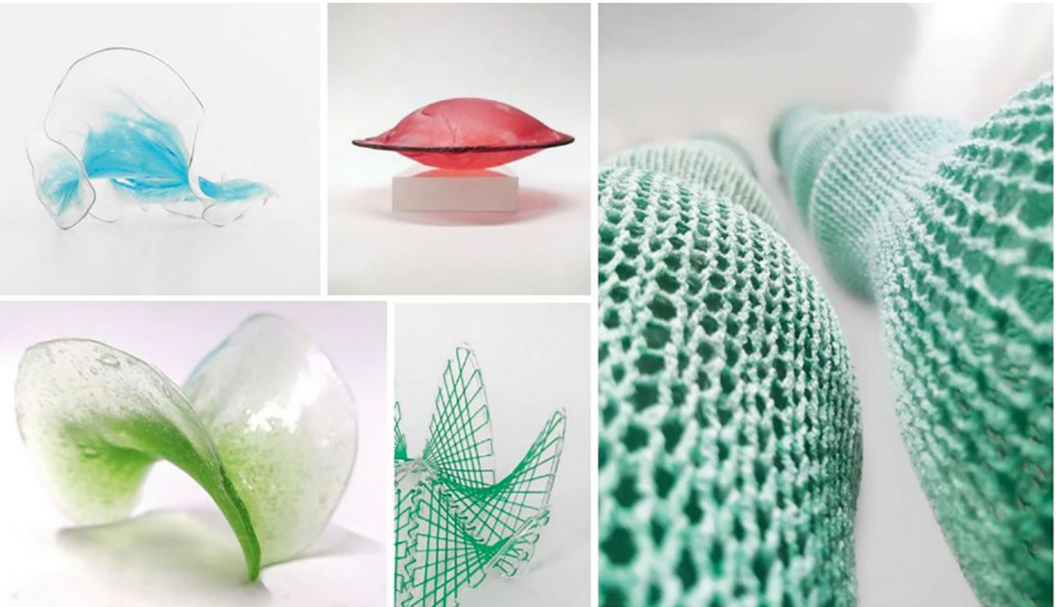
Figure 1: Different scale models made of alginate – from foils, threads, knitted structure to air cushions.
