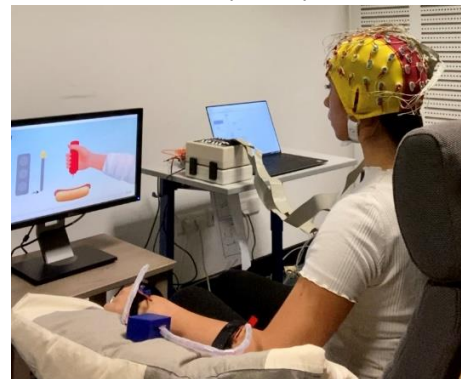
Figure 1. Three vibrotactile motors are located on the hand and the forearm. Their activation rotation frequencies and duration are synchronized and analogous to the visual feedback corresponding to four different levels of a grasping movement.
